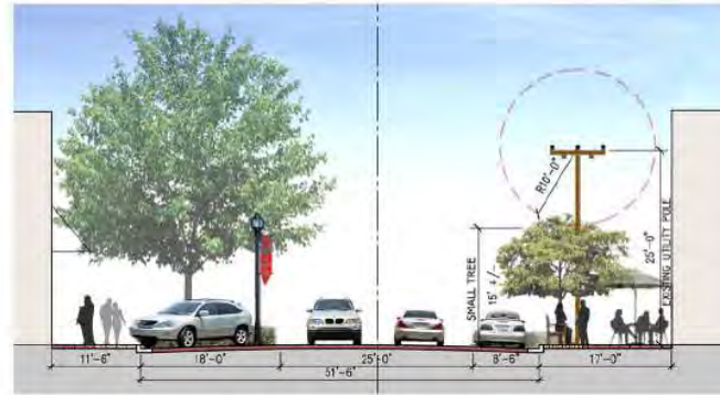
OPTION B - SMALL TREES AT OVERHEAD TRANSMISSION & DISTRIBUTION LINES ONLY, DIFFERENT SPECIES AT OTHER SIDE OF STREET
