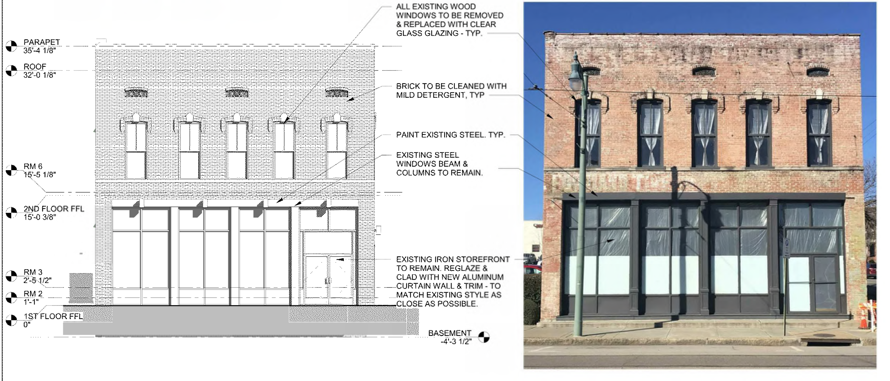
C3 EXTERIOR ELEVATION - EAST 1/8" = 1'-0"
