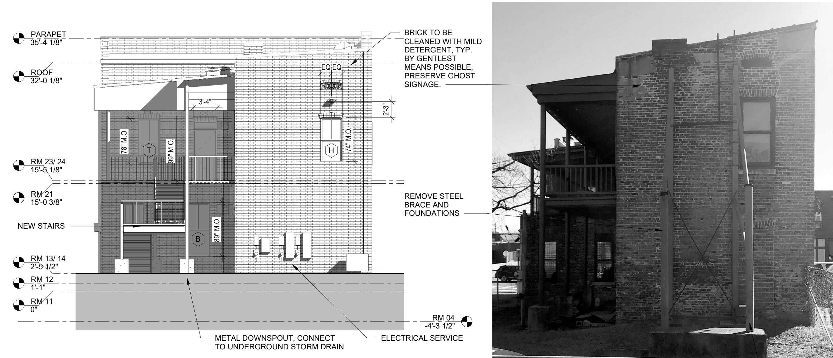
C1 EXTERIOR ELEVATION - WEST 1/8" = 1'-0"
