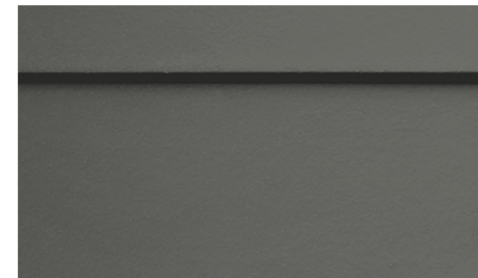
FC-1: FIBER CEMENT PANEL W/ BATTENS COLOR: SW-2849 WESTCHESTER GRAY
