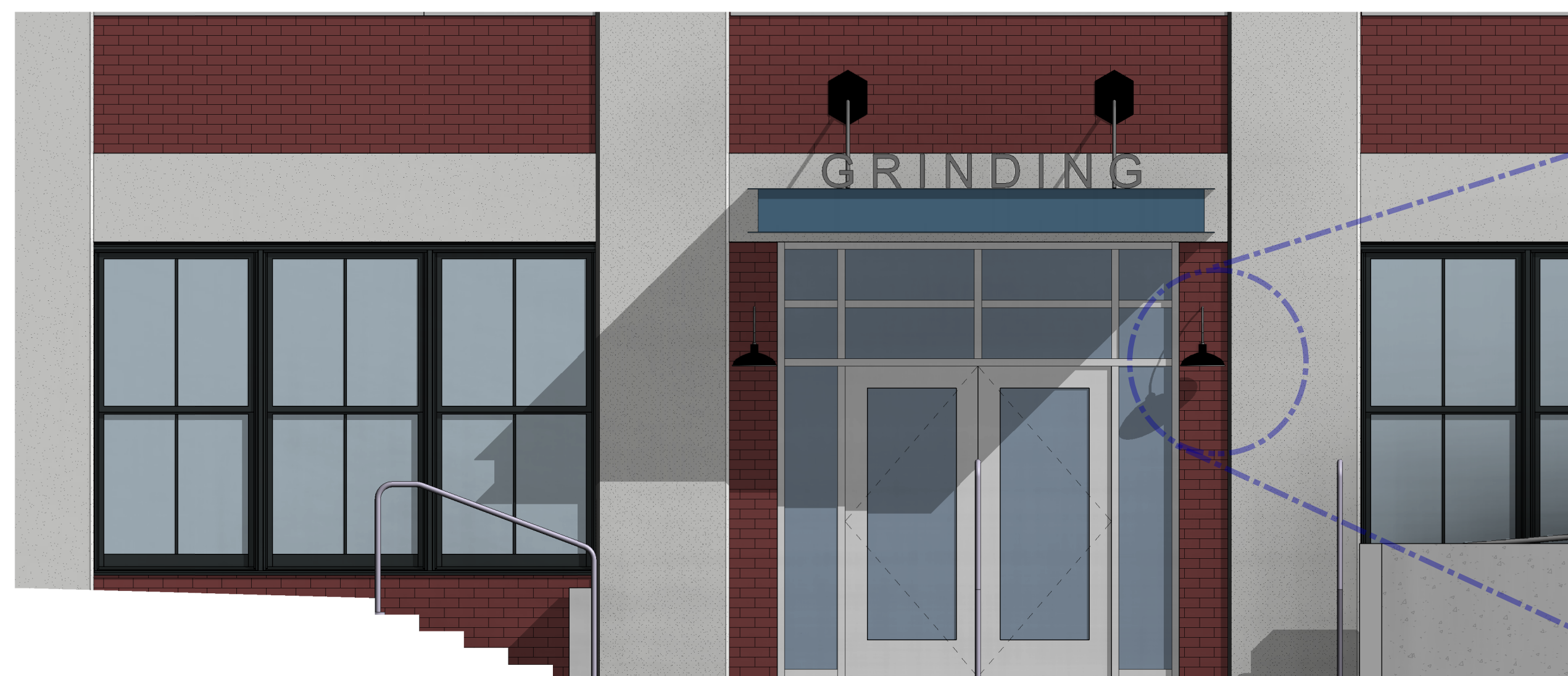
TYPICAL DOOR LIGHTING ELEVATION
