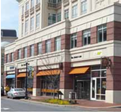
Incorporate a base, middle and cap into the building design where this is established along the street wall.
