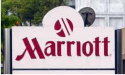
If internal illumination is used, a system that backlights sign text only, as seen on the metal sign above, is preferred.
