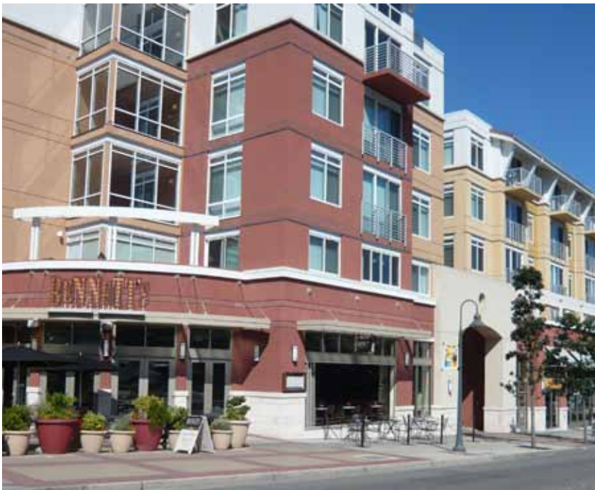
Variation in massing is important in large projects to convey a sense of human scale.
