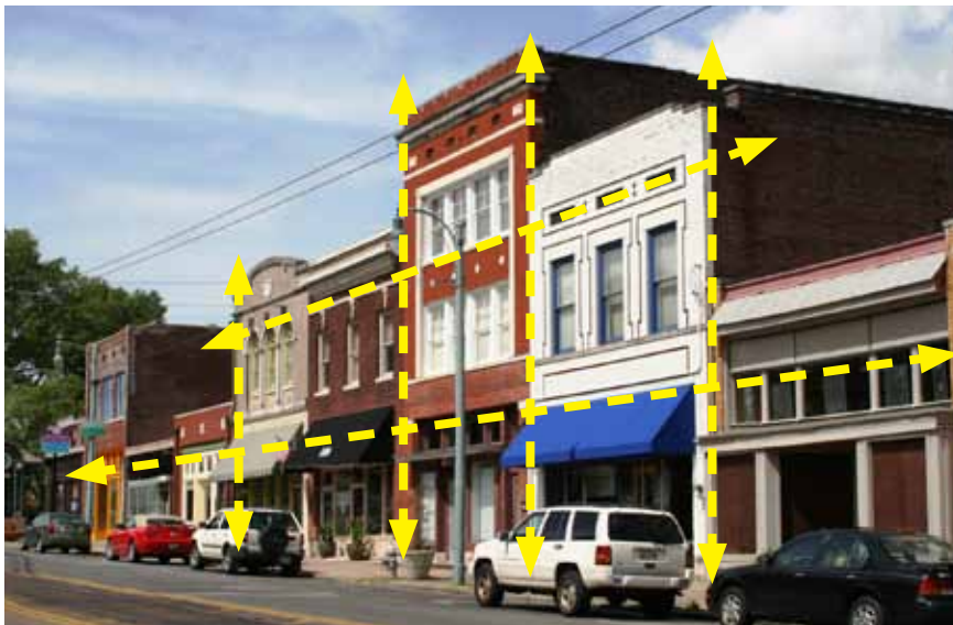
Features that convey a sense of relatedness include similar materials, the horizontal alignment of moldings and other wall features, and similar setbacks.
