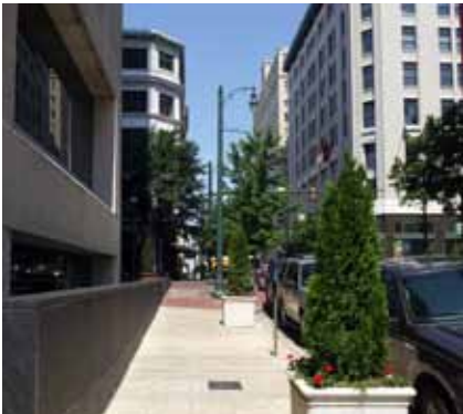
Since the Core is the densest area of Downtown, streetscape design should be urban in character with ample sidewalk width, street trees or planters, and pedestrian scaled lighting.
