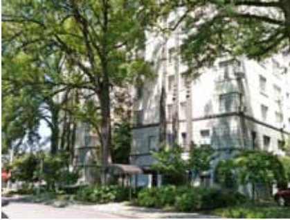
Planting or retaining trees helps to shade buildings and reduce solar gain.
