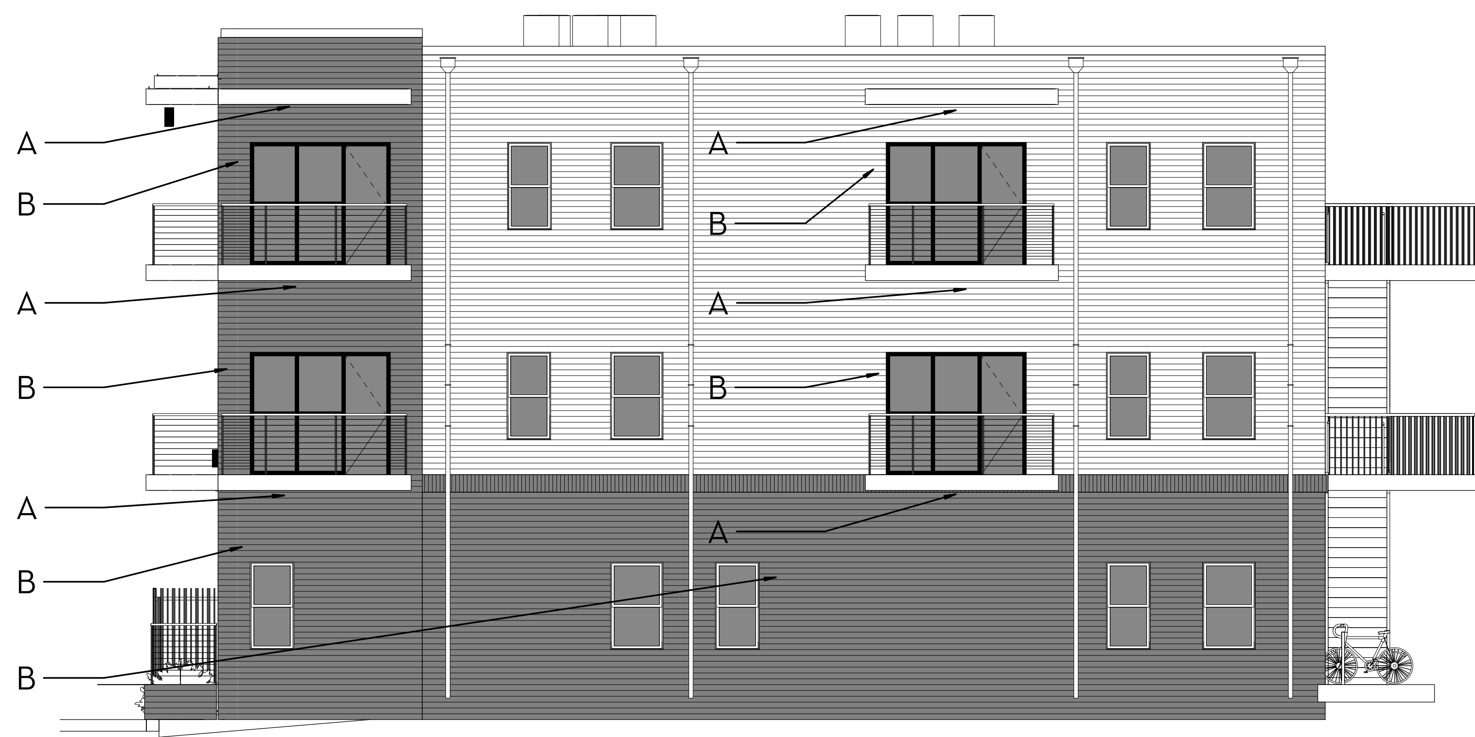
1 NORTH FACING ELEVATION LIGHT PLACEMENT 3/16" = 1'-0"
