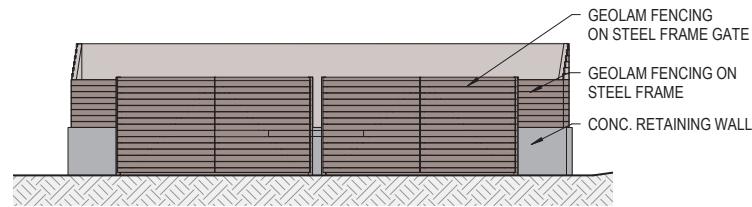
1 WEST ELEVATION- DUMPSTER ENCLOSURE SCALE: 1/16" = 1'-0"
