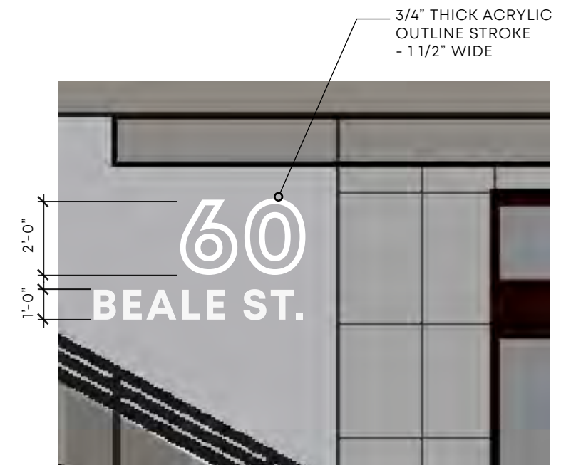
4 EAST ELEVATION - BUILDING ADDRESS Scale: 3/8" = 1'-0"
