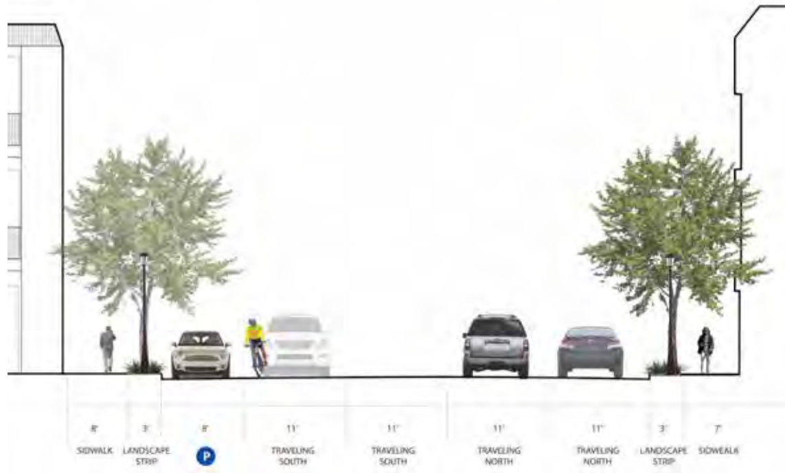
Proposed street section for Water Street, featuring shade trees and ground level plantings separating pedestrians from traffic, and narrower lanes to reduce vehicle speed
