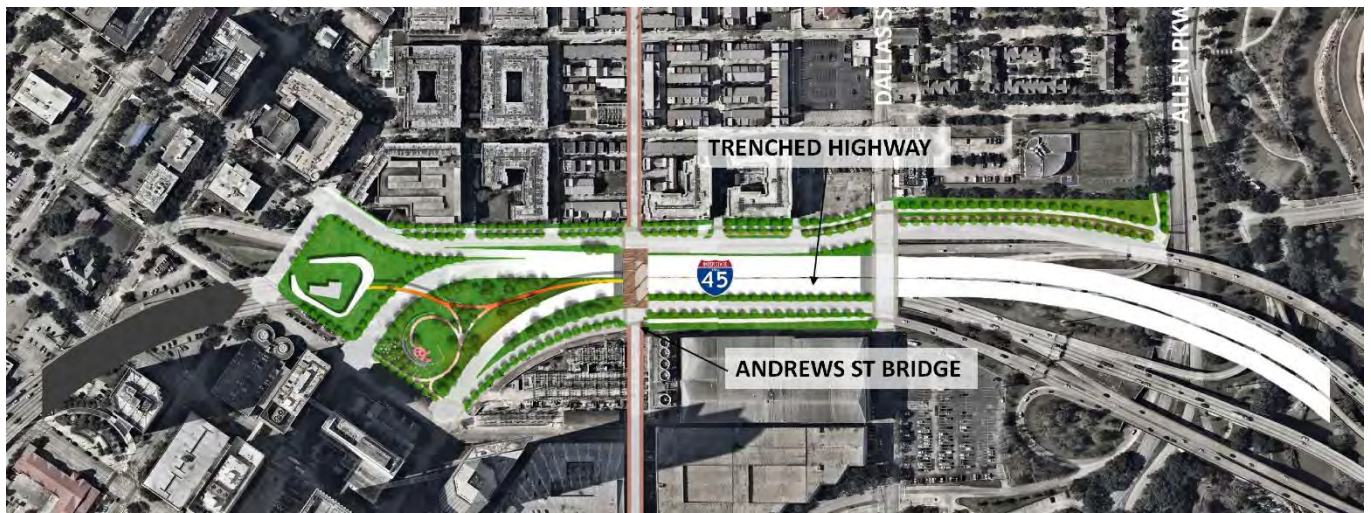
Proposed trenched Downtown Connector allowing Andrews St Pedestrian Bridge to extend through to Downtown
