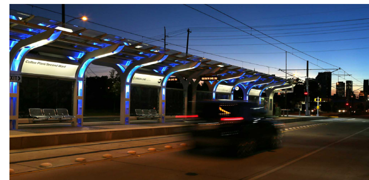
Houston, Texas: This preexisting rail stop provides a good example of a well illuminated station. The diffuse light from the columns add a pop of color to create a comfortable ambiance.
