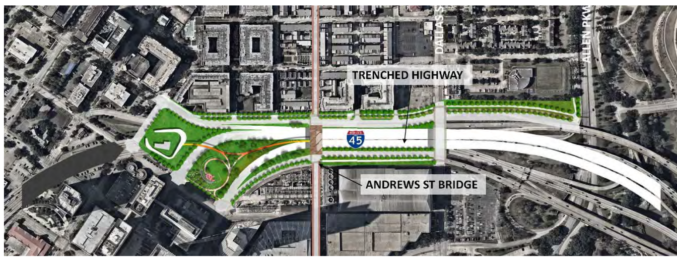
Proposed trenched Downtown Connector allowing Andrews St Pedestrian Bridge to extend through to Downtown
