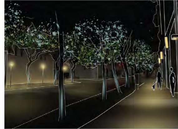
Relamp for Consistent Correlated Color Temperature
